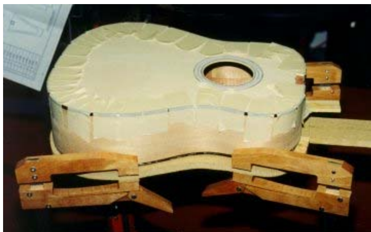
The completed bindings
